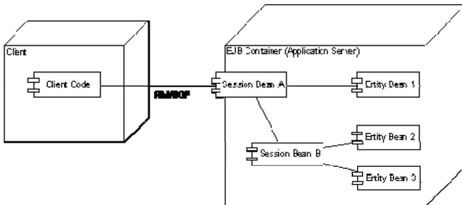
A façade has the advantage of simplifying the client's view of the remote application, since it hides most of the application's internal complexity. It can also make for reduced network traffic, if it provides bulk accessors to the clients – methods that can transfer a bulk of structured information in one single call across the network, rather than forcing the client to communicate with a bunch of different objects.
