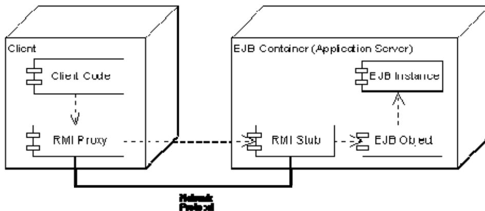
The diagram shows the architectural positioning of the EJB object relative to other major pieces. In the diagram, I'm showing the case of a remote client application, but you should keep in mind that there is always an intercepting EJB object, even when the method calls come from code in the same Container (another EJB, for example).
